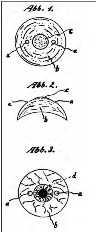
Figure 21-12 Extract of the Müller-Welt patent on contact glasses with perforations. This patent, registered in 1935, covers the principle and production of perforations in the scleral part of contact glasses intended to favor circulation and exchange of tears and avoid excessive adhesion of the glass. The orifices can be placed at a greater or lesser distance from the limbus, but always in the horizontal axis of the glass. (Mueller-Welt Gebr., 1935a)
