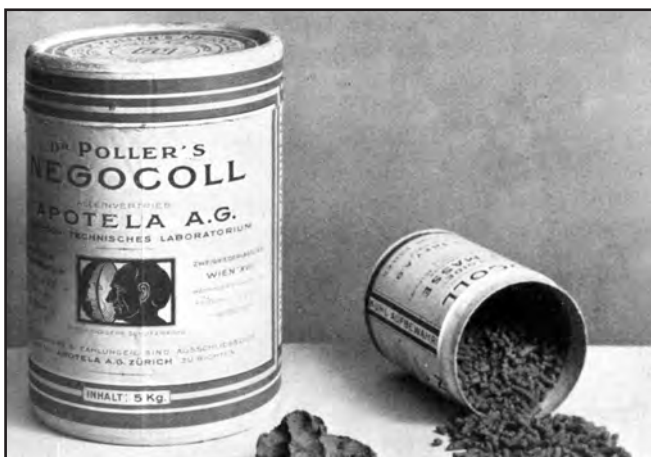
Figure 21-4 Poller's Negocoll. A 5 kg box and a 1 kg box of Negocoll. You see the small, mushy crumbs of the versed content of the box. Beside a small mass aggregative Negocoll, as obtained by the pressing with hand. (Poller A., 1931)
