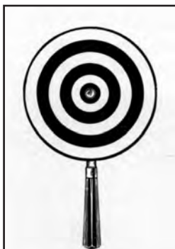
Figure 29-44 Placido's Disc (1882) The disc with concentric rings described in 1882 by the Portuguese ophthalmologist Antonio Placido was large in size. It was provided with a holding handle and possessed in its centre an orifice for observation of deformation of the rings reflected from the corneal surface. Subsequently, the Placido principle was followed by less bulky devices with different designs. (Placido A., 1882)
