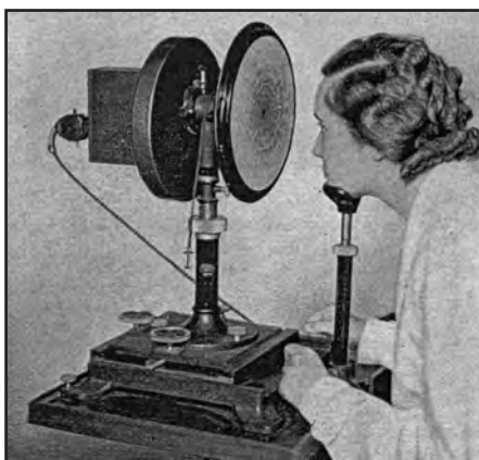
Figure 29-46 Zeiss-Fischer "Corneal Reflectograph" Designed by Fischer and manufactured by Zeiss, this "Corneal Reflectograph" was used for the study of corneal deformations after cataract surgery in order to provide a photographic image of corneal topography. (Fischer FP., 1928, 1932b; Hartinger H., 1932b)
