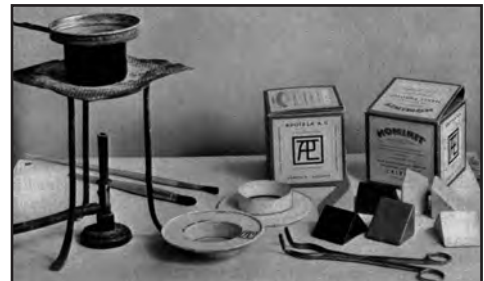
Figure 29-23 Products and utensils for Negocoll molding of objects, tissues and organs. In this figure, Poller illustrates the products and utensils necessary for Negocoll molding: a Bunsen burner with tripod, bowls and containers, forceps for manipulations, Hominit and Celerit prisms. (Poller A., 1931)
