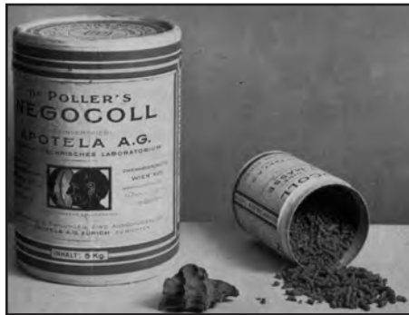
Figure 29-22 Poller's Negocoll for the molding of objects, tissues and organs. Poller's Negocoll was marketed by 'Laboratoire Technique Apotela A.G.' (Zurich, Switzerland) in metallic boxes of 5 kg and 1 kg. It was presented in the form of granules and could be modeled by pressure from the hands. (Poller A., 1931)
