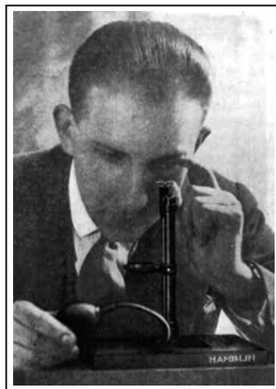
Figure 23-2 The Hamblin apparatus for insertion of a contact glass (1932). The apparatus for insertion of a contact lens consists of a cup-shaped rubber sucker supported on an upright standard which is fixed into a base-block. A small glass tube of narrow bore is fitted into the lower end of the sucker; to the other end of the glass tube is attached a small pressure bulb. Halfway up the standard is fixed a plane mirror, which may be rotated to left or right.
