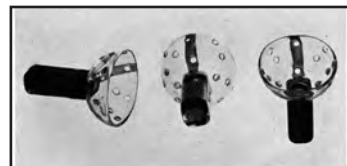
Lower figure: In the new plastic casting shells the wall is pierced with multiple perforations about 1 mm in diameter. These perforations, in conjunction with the hollow handle, allow the excess Moldite gel to escape. (Obrig T.E., Salvatori P.L., 1957)
