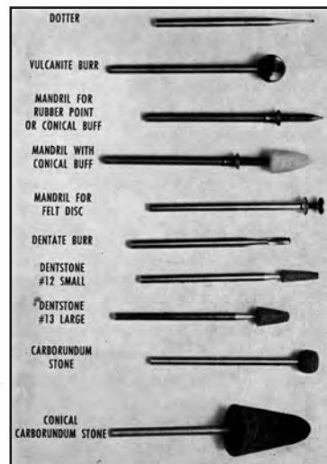
Figure 25-8 Tools used in fitting the 'Solutionless Lacrilens'. The lachrymal openings are drilled through the lens with a dental burr. The position of the hole should be in line with the vertical center of the corneal portion. The channels are ground from the bottom of the lachrymal vent upward and flaring outward across the entire lower corneal junction. The broad junction along the lower corneal limbus must be carefully blended. If the situation demands, the lens must be reduced in size. (Obrig T.E., Salvatori P.L., 1957)
